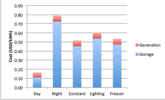
Fig. 3. Cost of electricity for different load profiles using Baseline inverter and battery system and hypothetical and measured loads. Storage costs are the dominant cost in each of these systems.
