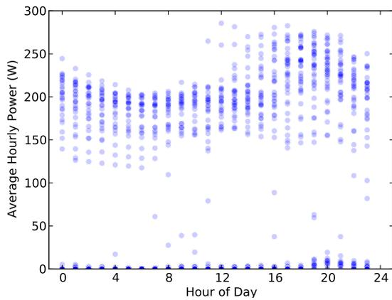
Fig. 7. Circuit with freezer. Each data point is the hourly load for a single day. The absolute variation in power is still significant but the ratio between high and low use is lower.
