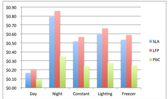
Fig. 5. Cost of electricity for different battery chemistries.
