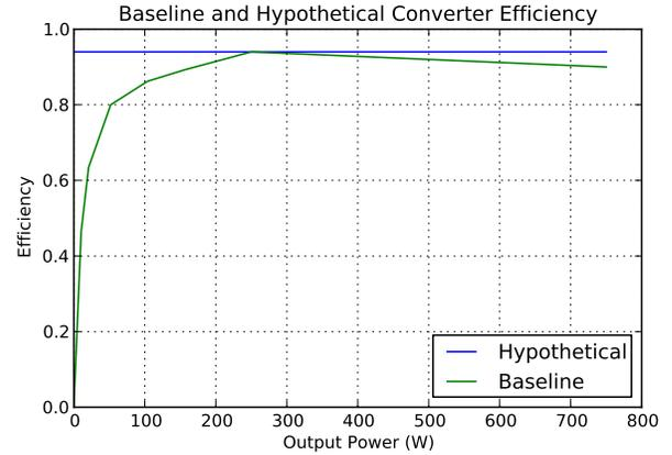
Fig. 2. Efficiency curves for baseline and proposed system. The proposed is a hypothetical system that has uniform efficiency at all power output levels.
