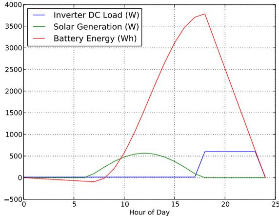
Fig. 1. Time series of simulation. The DC load of the inverter is plotted along with the solar generation as a function of hour. The solar panel size is adjusted until the battery energy at the end of the simulation is the same as the start value.
