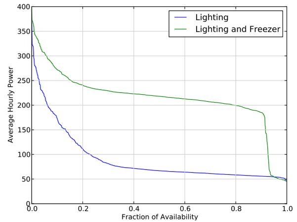
Fig. 8. Load duration curve for two typical microgrid systems, including metering, computing, and computation. Inverter and charge controller consumption is not included. One system includes a significant daytime refrigeration load, while the other does not.
