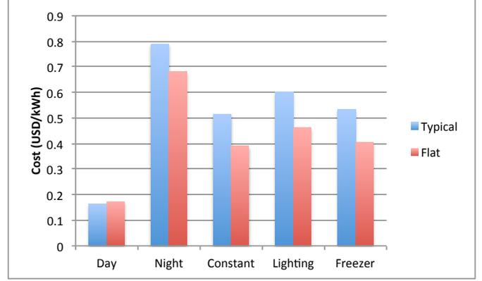
Fig. 4. The hypothetical “Flat” inverter efficiency curve results in a modest reduction of electricity cost.
