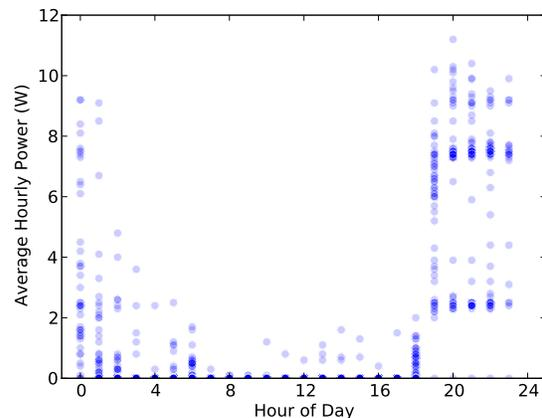
Fig. 6. Customer exhibiting two bulb lighting load. Each data point is the hourly load for a single day. Multiple days are superimposed. Points are transparent so that frequent measurements appear darker. This customer displays two common evening power levels corresponding to the use of one or two lightbulbs. This not that this customer has very small power use during the day.
