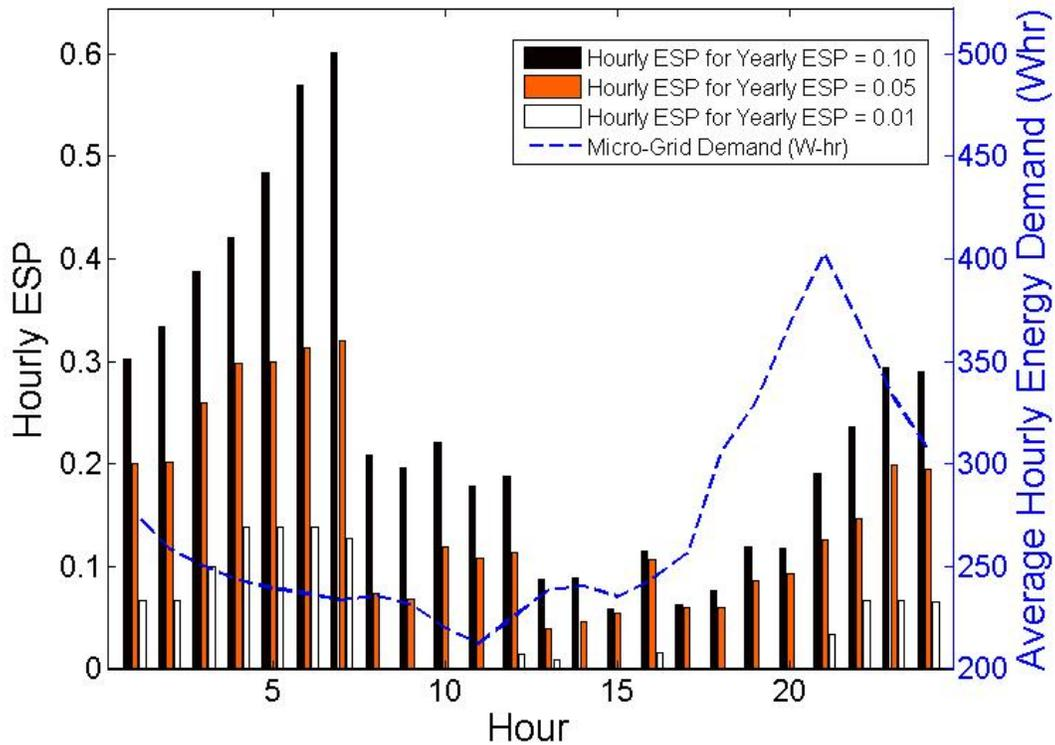
Figure 4: Bar plot of hourly *ESP* during the month of August. As indicated in the legend, the different bar column types are for micro-grids with Annual *ESPs* of 0.10, 0.05, and 0.01. Superimposed on the bar plot is the average hourly demand in Whr. The underlying model relies on the weather profile of Segou, Mali. The PV and battery composition of each micro-grid design is listed in Table 1.
