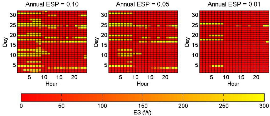
Figure 5: Maps of energy shortfall,  $ES$ , at an hourly resolution for the month of August. From left to right, subplots are for Annual  $ESP$ s of 0.10, 0.05, and 0.01. The underlying model relies on the weather profile of Segou, Mali. The PV and battery composition of each micro-grid design is listed in Table 1.
