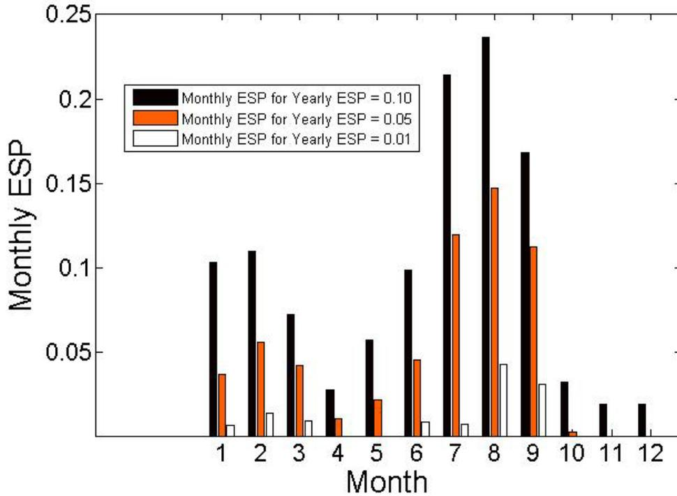
Figure 3: A bar plot of monthly *ESP* given annual *ESPs* of 0.10, 0.05, and 0.01. The underlying model relies on the weather profile of Segou, Mali. The demand data is for the micro-grid with a freezer base load. The PV and battery composition of each micro-grid design is listed in Table 1.
